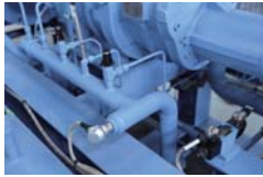
Original oil injection system
