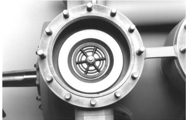
Fig.153: Top view of discharge valve assy
