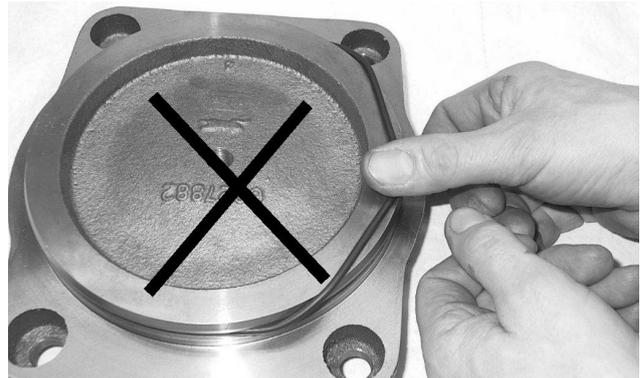
Fig.179: WRONG WAY OF MOUNTING
